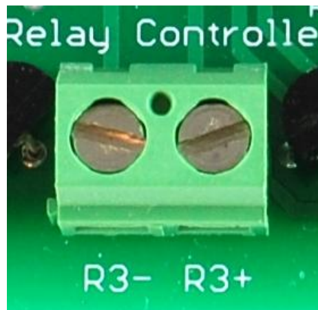
Figure 1. Relay Connection Terminal
